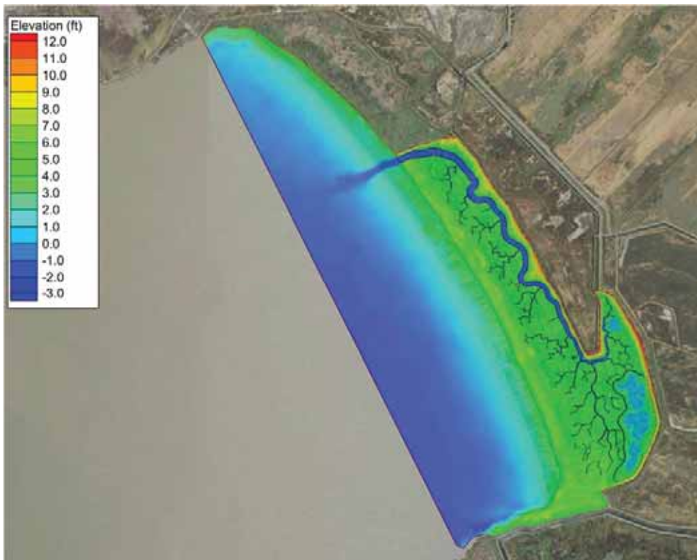
Figure 4.4: Future conditions model topography, note fully developed entrance channel and tidal mudflat channel
