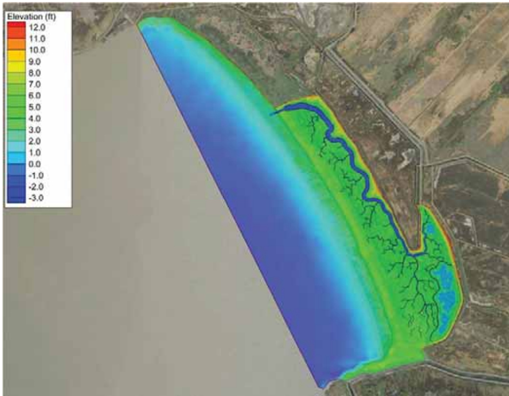
Figure 4.3: As-built model topography, note undersized entrance channel and no tidal mudflat channel
