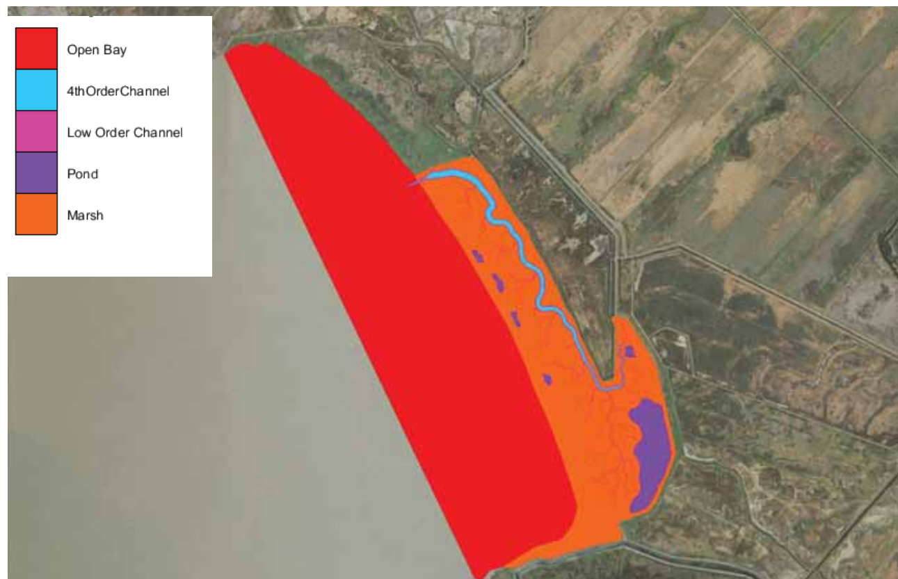
Figure 4.1: ADH model extents and material types for project conditions
